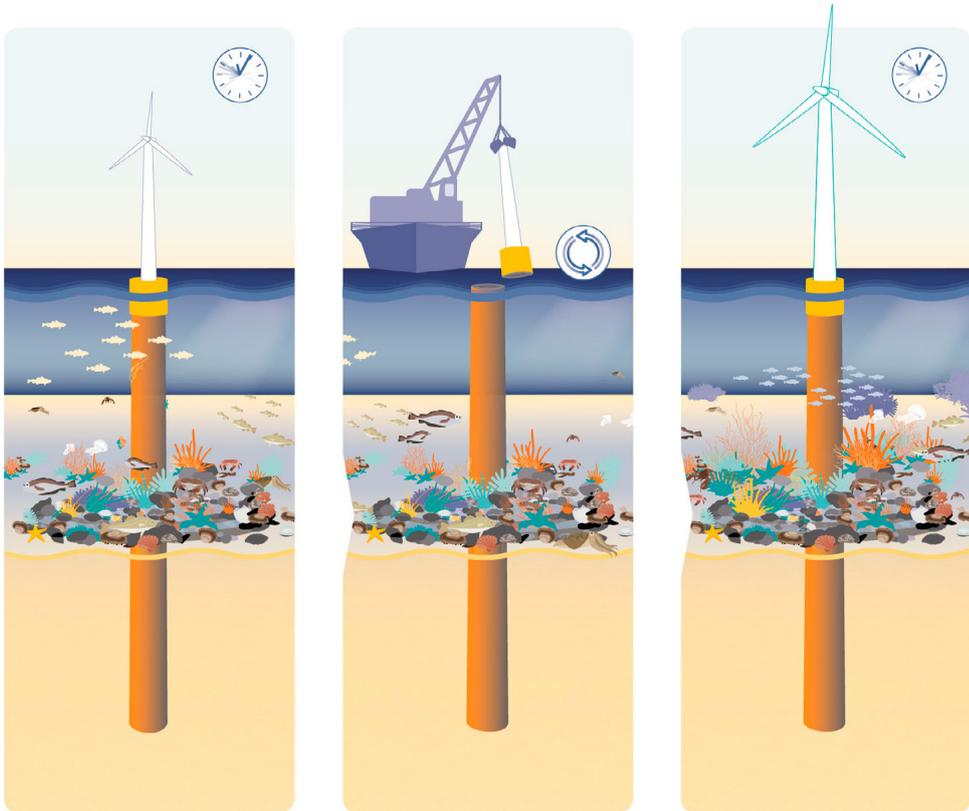
Figure 3: a schematic representation of life span extension of the wind turbine and the reuse of its foundation. The foundation is designed (overengineered) in such a way that it is suitable for a larger, modern turbine.
